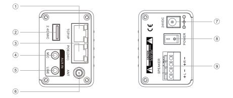
1. 10M/100M network port, used to connect to LAN, it is recommended that customers use standard network.
