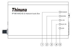
1. POWER indicator light, when the device is powered on, the indicator light is always on; when the network location is turned on, the indicator light flashes at a fixed frequency.
